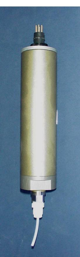
The SBE 29 pressure sensor, used on our SBE 25 SEALOGGER CTD, is a modular sensor consisting of a mechanical strain-gauge pressure transducer with thermistor temperature compensation. The SBE 29 measures absolute pressure in one of seven full-scale pressure ranges from 20 to 7,000 meters depth. The sensor elements and their interface electronics are modular and self-contained, providing easy installation, service, and calibration.
