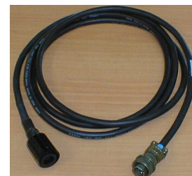
Deck Unit to 9plus test cable
