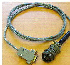
CDO Remote Out Interface test cable
