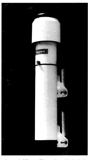
the column level reaches a maximum of 250 mm (50 mm of precipitation), the chamber automatically empties and the process repeats. Total precipitation can be tracked by a datalogger or recorder.
